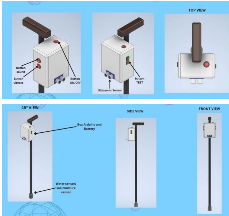
Figure 2. 3D drawing of a smart blind stick
