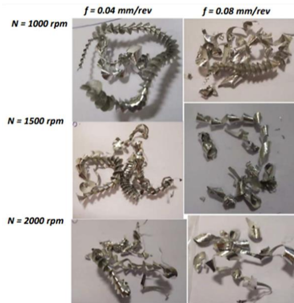
Figure 5. Example of chip formation under different spindle speeds and feed rates [8]
