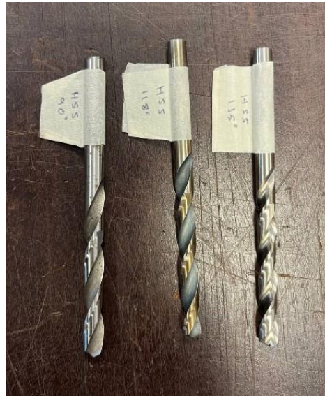
Figure 6. HSS twist drill bit with 3 different point angles of 90°, 118° and 135°
