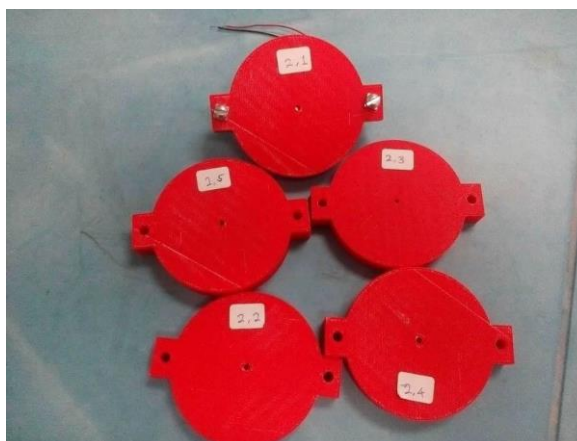
Figure 2: One of set synthetic jet actuator with different nozzle size and volume cavity
