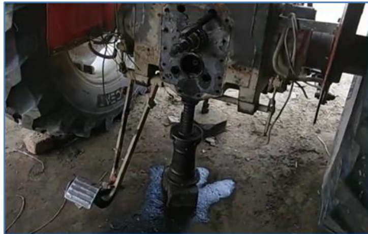
Figure 6: Jack stand used to hold the tractor during servicing work
