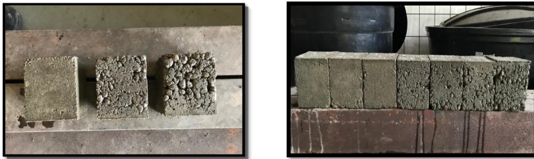
Figure 6: The surface texture of mortar cube of LECA mixture
