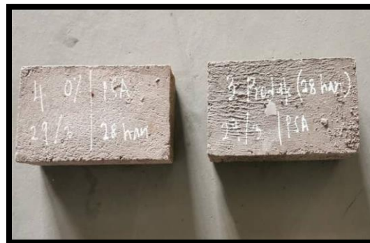
Figure 9: Final brick product with dimension 216mm x 103mm x 65mm
