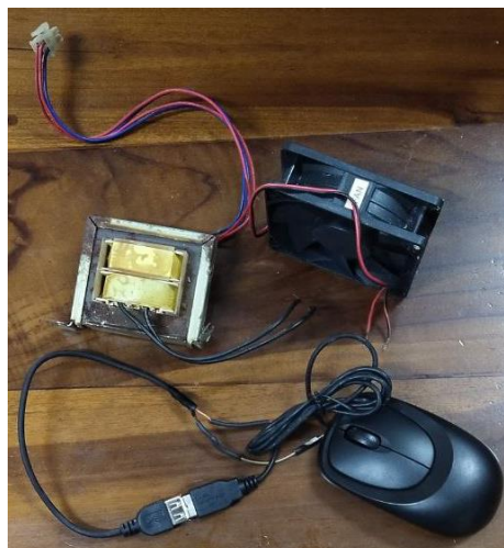
Figure 5. Output connected with 5 V DC and 12 V DC
