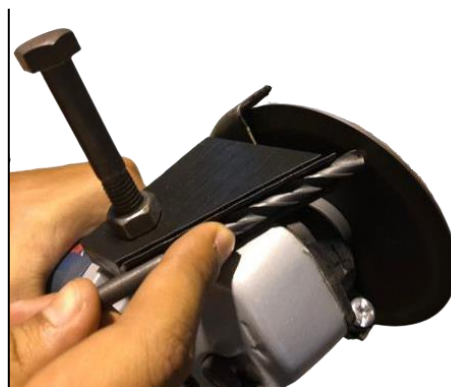
Figure 5. Drill Bit Sharpening Jig Attached on Hand Grinder Machine
